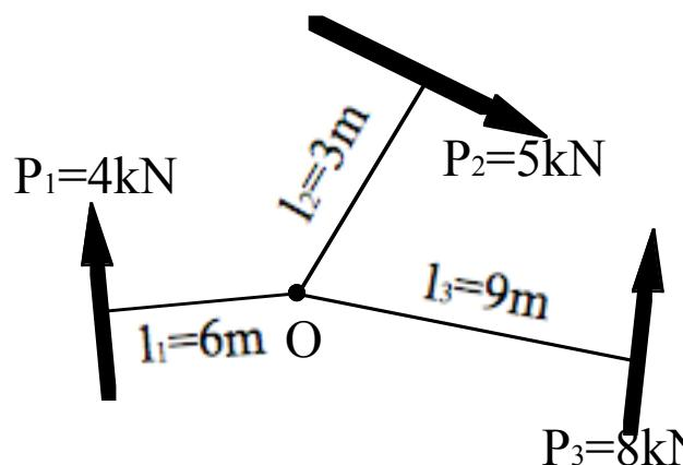
$$\begin{aligned} M &= P_1 \cdot l_1 + P_2 \cdot l_2 - P_3 \cdot l_3 \\ &= 4kN \times 6m + 5kN \times 3m - 8kN \times 9m \\ &= -33kN \cdot m \end{aligned}$$
