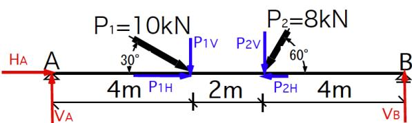
$$P_{1V} = P_1 \times \sin 30^\circ = 5.0kN, \quad P_{1H} = P_1 \times \cos 30^\circ = 8.66kN$$
