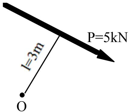
$$M = P \cdot l = 5kN \times 3m = 15kN \cdot m$$
