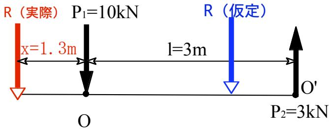
$$R = -P_1 + P_2 = -10\text{kN} + 3\text{kN} = -7\text{kN} \text{ (下向き)}$$
