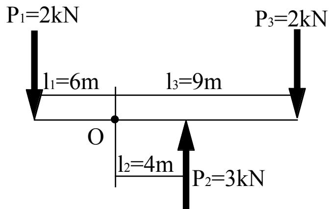
$$\begin{aligned} M &= -P_1 \cdot l_1 - P_2 \cdot l_2 + P_3 \cdot l_3 \\ &= -2kN \times 6m - 3kN \times 4m + 2kN \times 9m \\ &= -6kN \cdot m \end{aligned}$$
