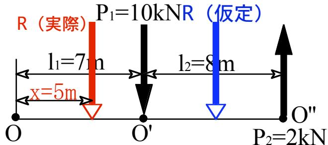
$$R = -P_1 + P_2 = -10\text{kN} + 2\text{kN} = -8\text{kN} \text{ (下向き)}$$
