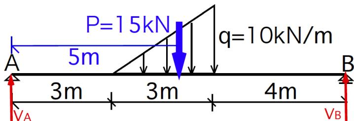
$$P = \frac{10\text{ kN/m} \times 3\text{ m}}{2} = 15\text{ kN}$$
