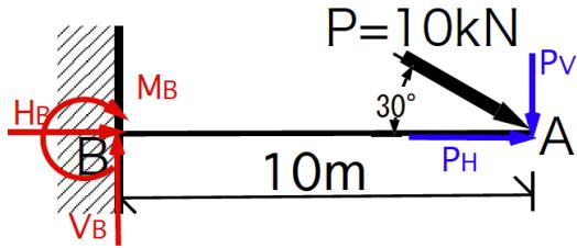
$$P_v = P \times \sin 30^\circ = 5.0\text{ kN} , \quad P_H = P \times \cos 30^\circ = 8.66\text{ kN}$$
