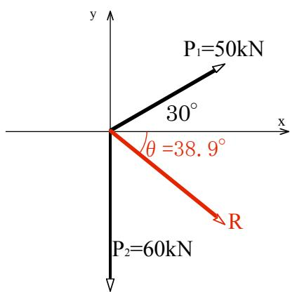
$$P_{1x} = P_1 \times \cos 30^\circ = 50\text{kN} \times \cos 30^\circ = 43.3\text{kN}$$
