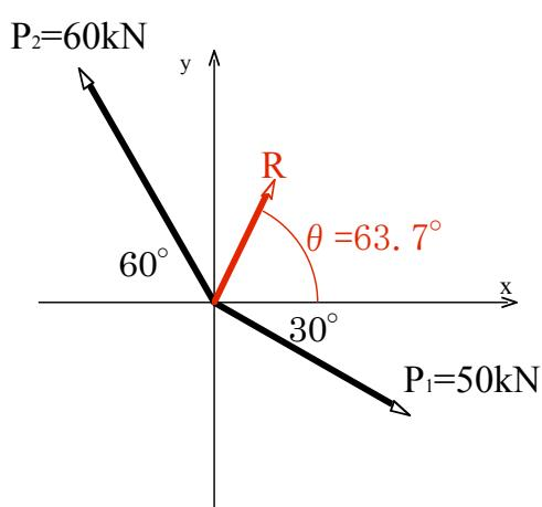
$$P_{1x} = P_1 \times \cos 30^\circ = 50\text{kN} \times \cos 30^\circ = 43.3\text{kN}$$
