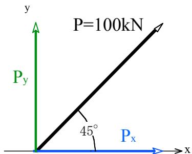
$$P_x = P \times \cos 45^\circ = 100 \text{ kN} \times \cos 45^\circ = 70.7 \text{ kN}$$
