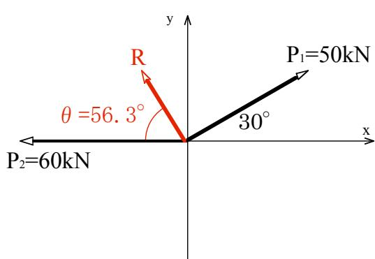
$$P_{1x} = P_1 \times \cos 30^\circ = 50 \text{ kN} \times \cos 30^\circ = 43.3 \text{ kN}$$
