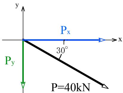
$$P_x = P \times \cos 30^\circ = 40 \text{ kN} \times \cos 30^\circ = 34.6 \text{ kN}$$
