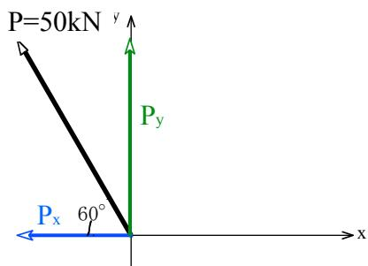
$$P_x = -P \times \cos 60^\circ = 50 \text{ kN} \times \cos 60^\circ = -25 \text{ kN}$$
